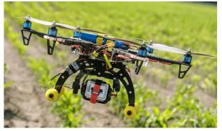
digital terrain, 3D model, vegetation and geometric map. The camera's imaging captures multiple data at one go that can provide crop health report, pinpointing location of pest infestation and water retention in different parts of the farm.
